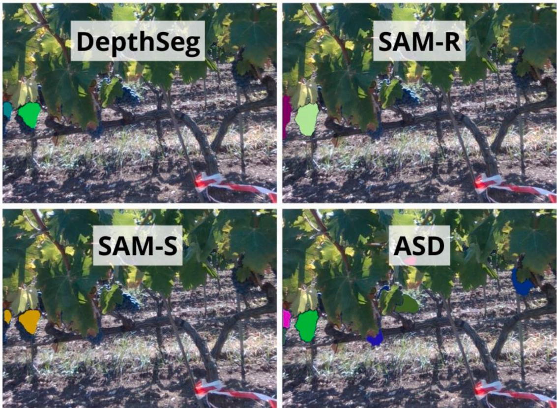
Fig. 17. Impact of Initial Segmentation Quality: The visual contrasts here highlight the dependency of DepthSeg, SAM-R, and SAM-S on the quality of initial segmentation and the superior performance of ASD in segment the scenes.
